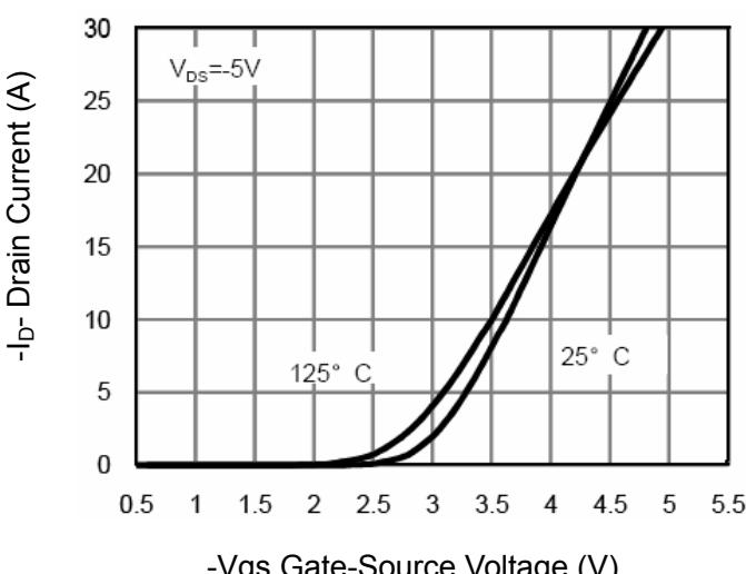
**Figure 2 Transfer Characteristics**
