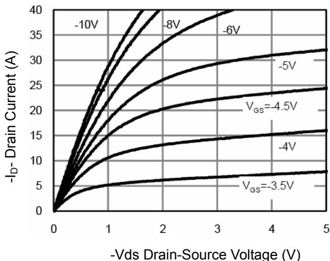
**Figure 1 Output Characteristics**
